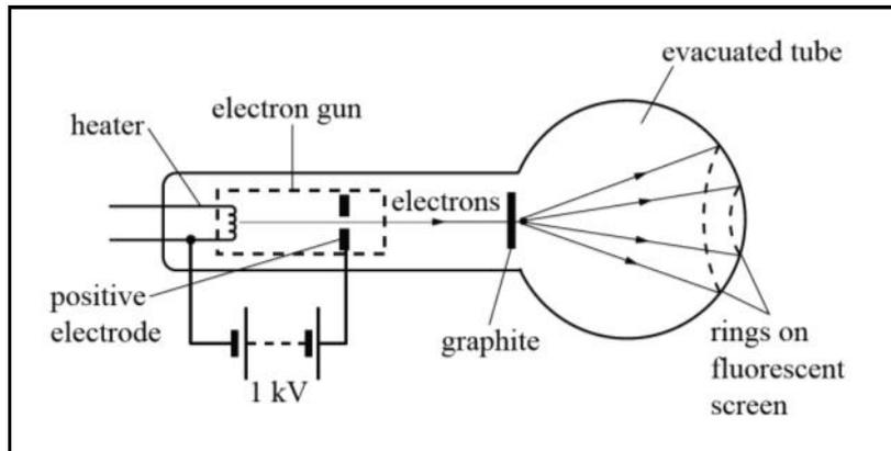
The electrons are accelerated to high speeds by the electron gun. These high speed electrons pass through a thin layer of graphite (carbon atoms) and emerge to produce rings on the fluorescent screen.
