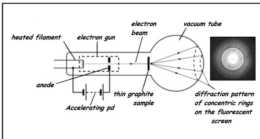
The apparatus shown above is used to demonstrate electron diffraction.
